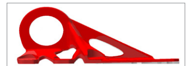
Distorted geometry after printing
