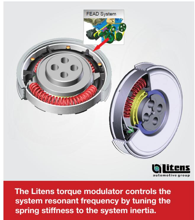
**The Litens torque modulator controls the system resonant frequency by tuning the spring stiffness to the system inertia.**
