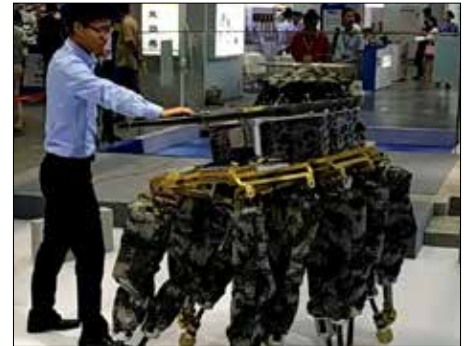
Robot balances itself after being pushed
