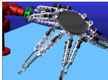
Adams simulation of Octopus robot closing a valve
