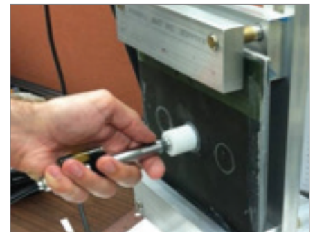
Figure 2. Performing QPD measurements on bonded carbon fiber reinforced composite laminates.
