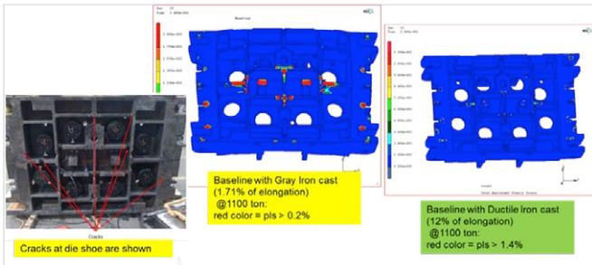
Figure 3: Total equivalent plastic strain plot of gray cast iron die shoe matches cracks seen in the physical die shoe while simulation of the ductile cast iron shoe indicates that cracking will not occur.
