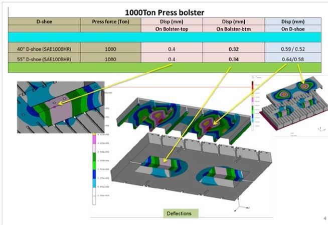
Figure 2: Results of the die bolster study show that the die bolster deflection is less than the die shoe
