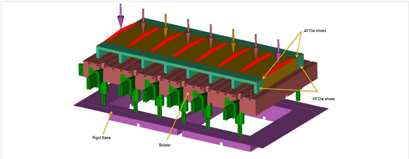
Figure 1: 1000-ton press die bolster model
