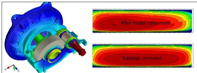
The more complex Romax model with FE housing (left), contact pattern after refinement matching the test rig results (top right), contact pattern after further optimisation (bottom right)
