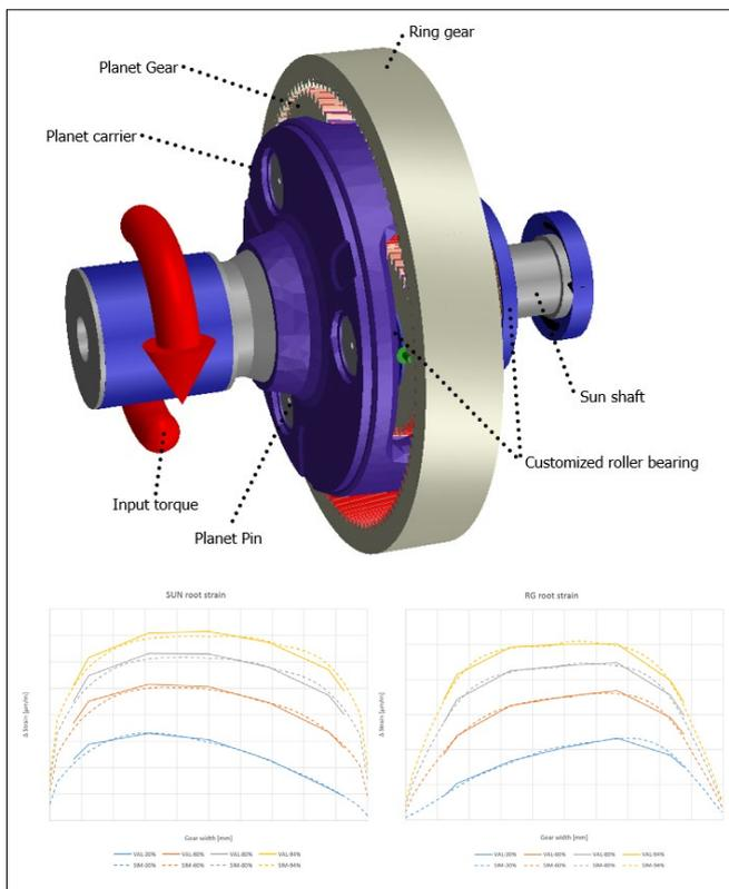
Top: Planetary gear stage design modelled in Romax Enduro; Bottom: Correlation of root strain values against mesh width of the sun (left) and ring (right) gears, showing measurement vs simulation at varying load levels
