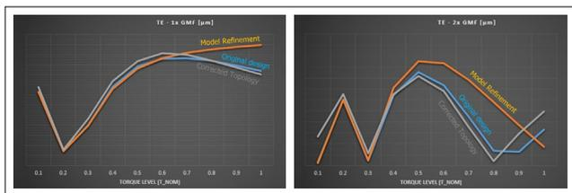
The original simple simulation model (blue) showed decreasing TE above 50-60% torque but the test rig actually showed an increase. After refinement, the simulation model (orange) matched this observation, and some further optimisation of the more complex model improved the TE (grey). Left – first order harmonic, right – second order harmonic
