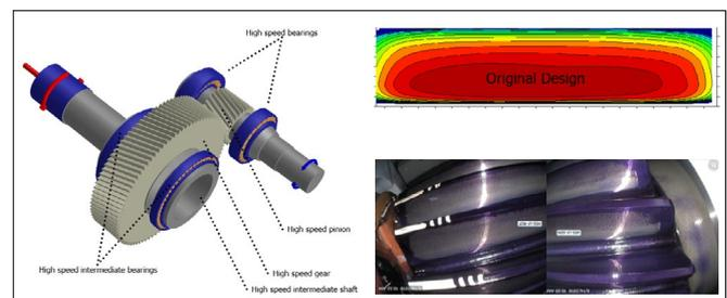
Although the very simple Romax model (left) showed a central contact pattern (top right), the test rig showed more loading on the left side of the gear than the right (bottom right)
