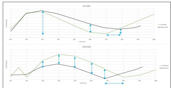
TE results: simulation vs test rig (1st and 2nd order plots)
