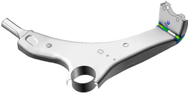
Elasto-plastic simulation of an automotive link arm
