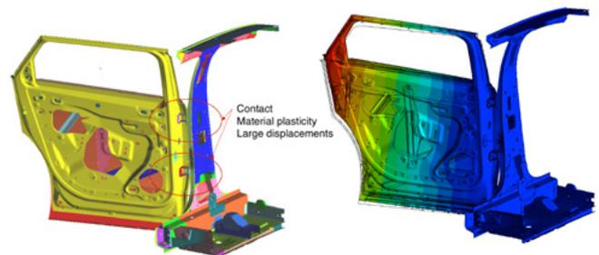
SOL400 simulation of partial car body & rear door, image courtesy of PSA
