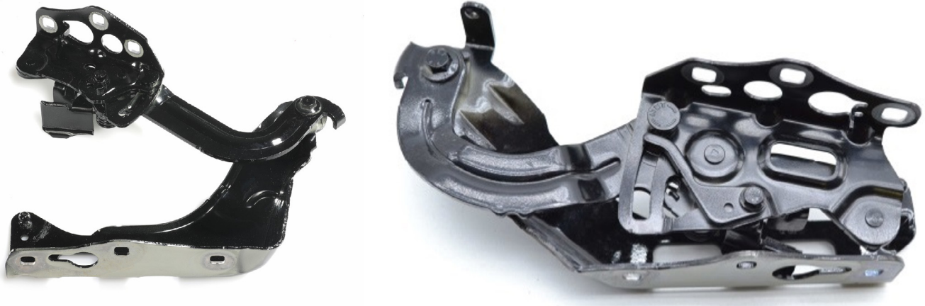
Weight-intensive, conventional design of an engine hood hinge with a high component count
